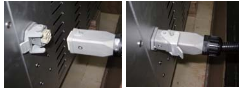
② Insert it to the connector on the right bottom side of the kiln.
